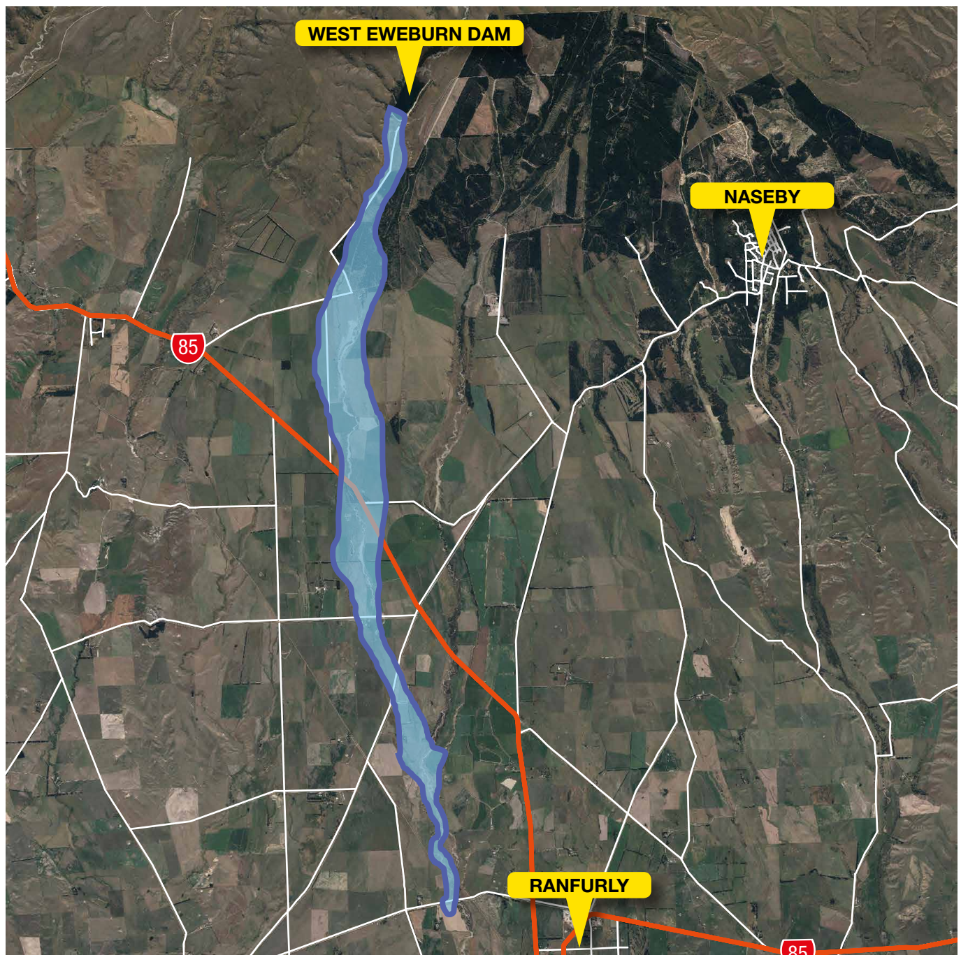
Indicative Only – Otago Irrigation Dam Break Hazard Assessment, Circa 1989
